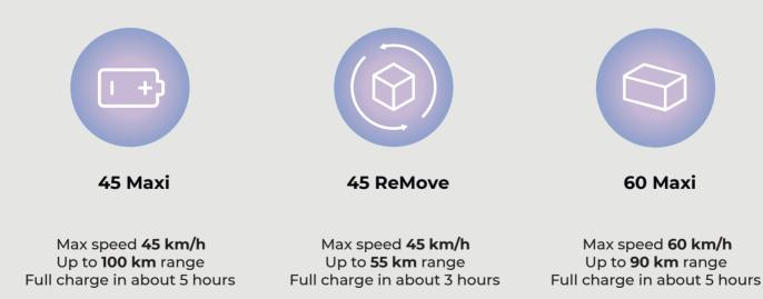
All our batteries are 5.5 kWh Li-ion and their charging absorption have a maximum of 1 kW.
